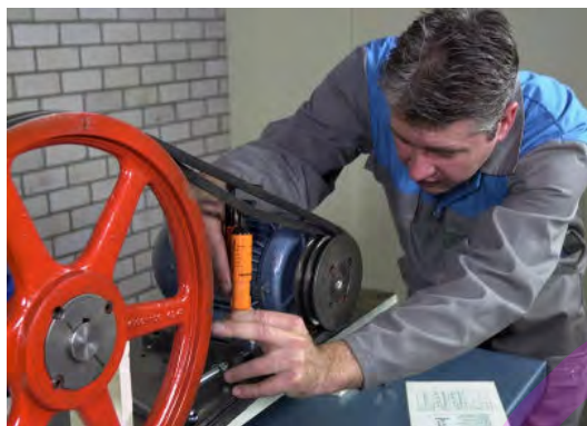
Spanning in riem controleren
